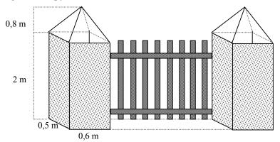
Determine the volume of cement needed to make up the two pillars.
