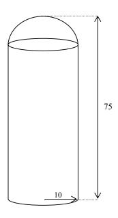
Calculate the total exterior surface area of the tank.
